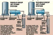
**Well Storage Tank** – a tank in a water well system that can help store water to increase the available water supply
