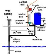
**Well Pump System** – a household pump system that pressurizes and injects water from a cistern or a well into the home's plumbing system
